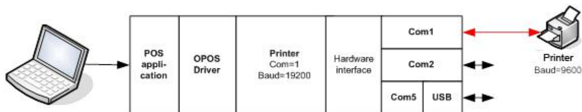
Figure 9. Incorrect configuration – baud settings do not match.
